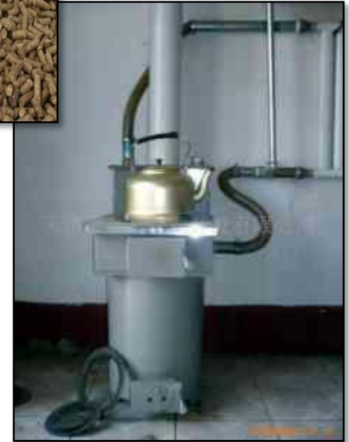
Biomass pellet gasifier stove for cooking & heating
