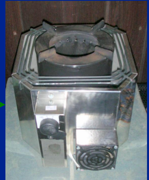
Gasifier Stove with Electric Blower (battery recharged with cell phone charger)
