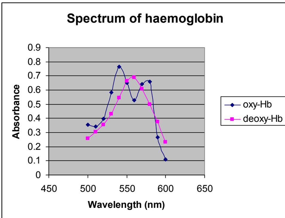
This seemed to be done rather well, with most students remembering to re-zero the machine against water for each wavelength studied. This needs to be done as the spectrophotometer lamp does not put out the same level of illumination at every wavelength. The graph below shows typical data obtained from a session. It can be seen that oxy-haemoglobin has two main peaks, at 540 and 577 nm (if the investigation had been extended, you may also have found a peak at 412 nm).
